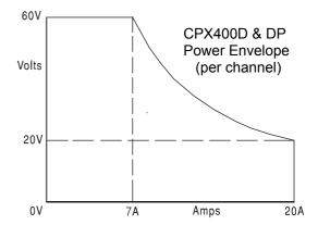
**Operating Ranges:** Four selectable ranges: 60V/20A, 60V/7A, 20V/20A and Custom Limits.
